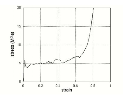
In compression, SAF exhibits a long plateau region in stress over very large strains, meaning it can absorb energy while exerting a constant force. SAF can be produced in a range of densities allowing for the force or energy absorption requirements to be tailored to the application.
